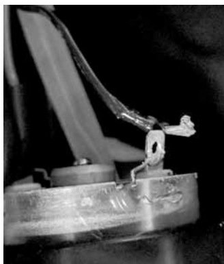
Pumb of Keurig showing wire (black) dangling near the ring that it used to be soldered to
